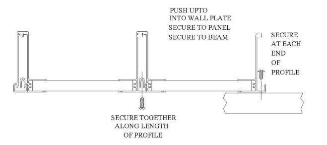
At right hand end use final single End Closure to complete appearance, fix through angled edge as previous, along length.
