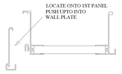
Secure along length to previous aluminium profile. At each end secure to wall plate and support frame.
