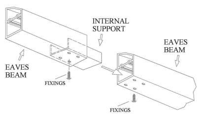
To obtain good water flow ensure the eaves beam is positioned (see diagram) with the slope away from the wall.
