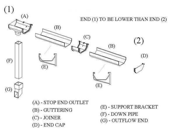
Decide which end of the canopy the down spout is to be (where the flow of water won't be a problem). This will then determine the position of the "Stop End Outlet". Blank off relevant end.
