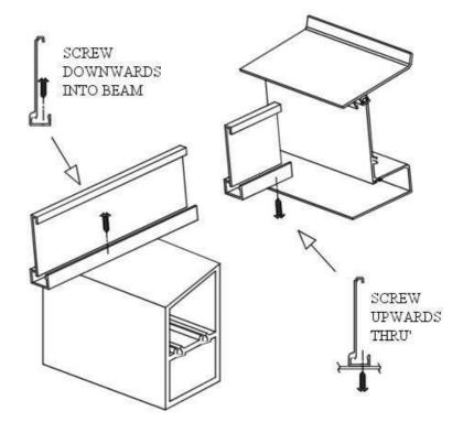
Each glazing panel has a polycarbonate protrusion of approximately 25mm this needs to be fed into the wall plate to provide a watertight seal. Ensure panel pushed fully into wall plate, front edge should be level with previously fixed part.
