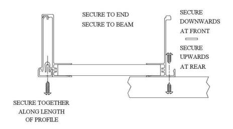
Lift one pre-assembled panels on to the roof and locate onto the previously fixed Aluminium profile.
