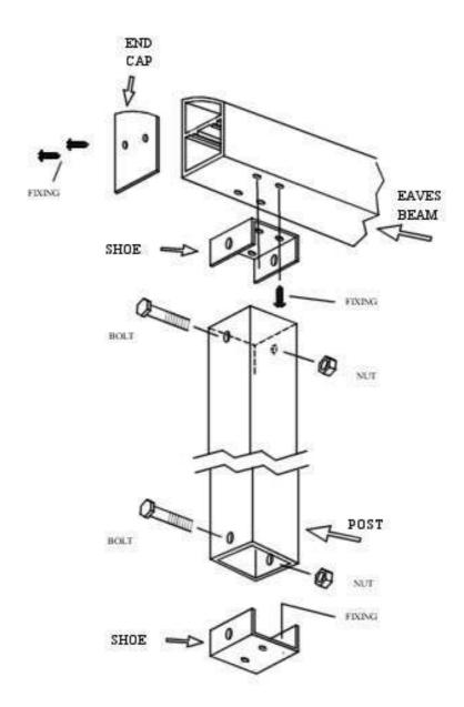
On longer lengths Eaves beams will have to be joined, see diagram right.
