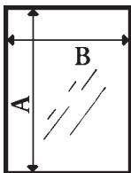
1. Measure the existing window pane, vertically (measurement A) and horizontally (measurement B). **This is the visible glass only and does not include any frame.**
