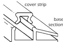
When use of the windows is required we suggest the glass is installed externally. When using SUPERGLAZE ensure there is at least 20mm of flat mounting surface around each side of the glass to take the fixings.
