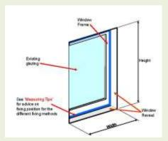
We offer a free cut to size service. Just give us the dimensions at time of order. Our saw cuts to a tolerance of +/-3mm. When considering on where to place/fit the secondary glazing panel please consider the following.
