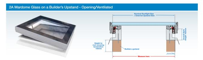
The direct fix kerb is supplied as standard to facilitate fixing to a builder's upstand if ventilated or opening options are specified.
