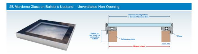
Mardome Glass is available as a glazing only, unventilated non-opening unit for fitting to existing builder's upstands and are mechanically fixed through the side of the profile into the vertical face of the upstand.
