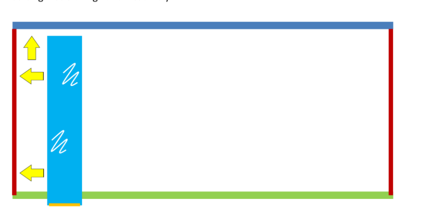
Inserting first Glazing Panel Assembly
